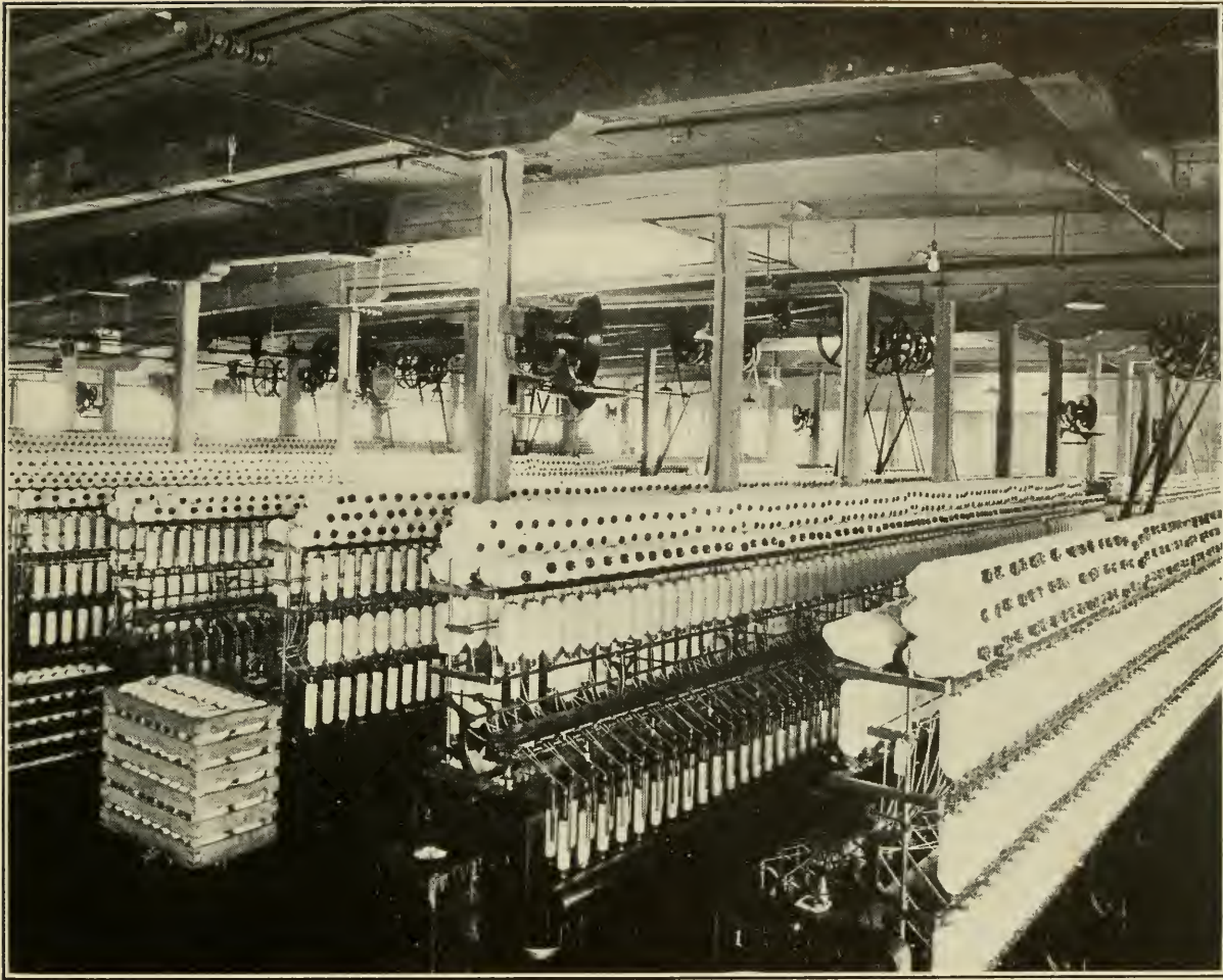
SECTION OF ROVING FRAMES IN CARD ROOM
